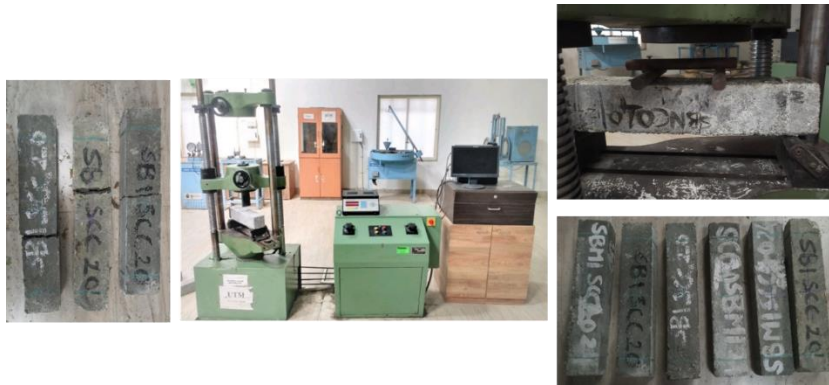
Fig. 6 Arrangements of loading and specimen for Flexural strength test
