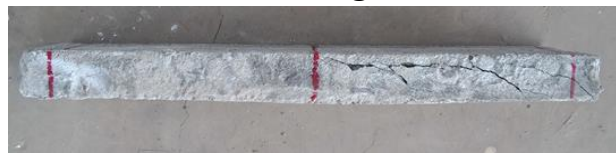
b. Shear Failure
