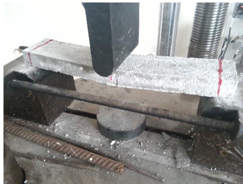
Figure 5. Flexural test of ferrocement panel
