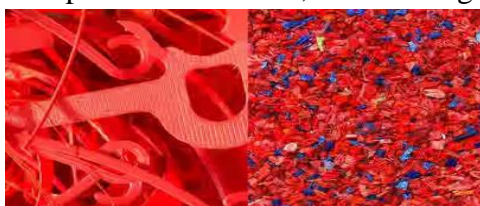
(Shredded state of a 3D printed Products) (Figure-1)
