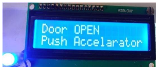
Figure 7 Output of the system, when door opened.
