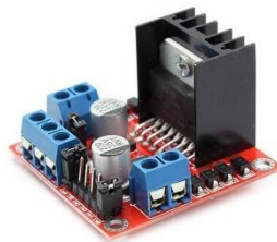
Fig.10. DC Motor Drive
