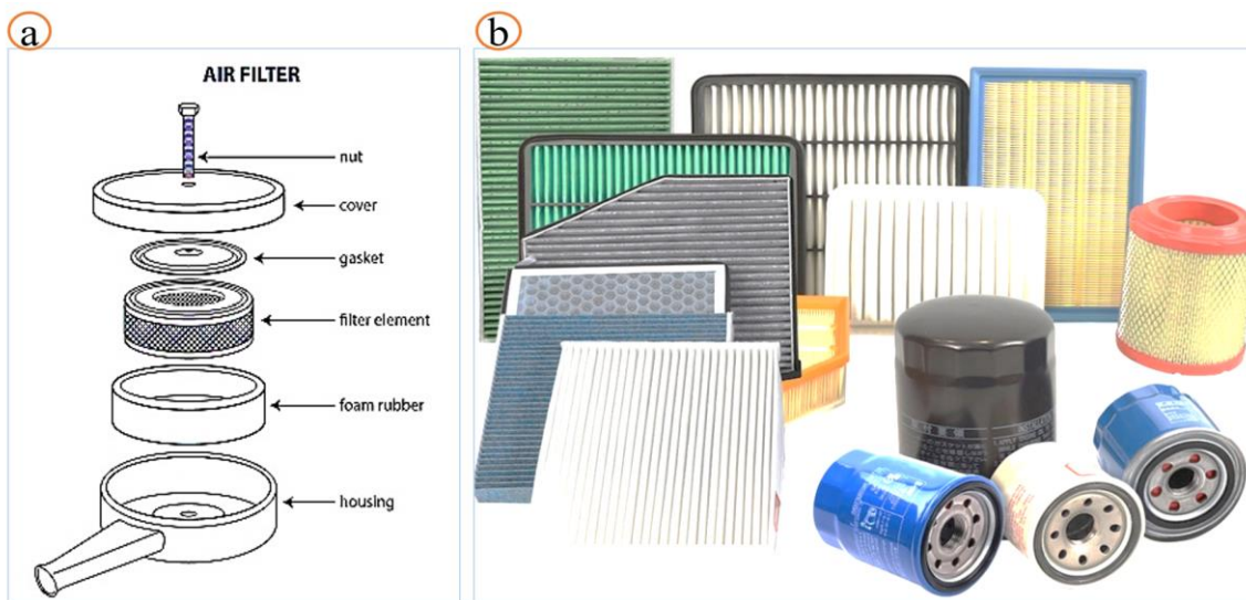
Figure 1: (a) illustrate the different parts of car air filters. (b) exhibit the different type of car air filters that is utilized for car cabin, engine and oil filtration.
