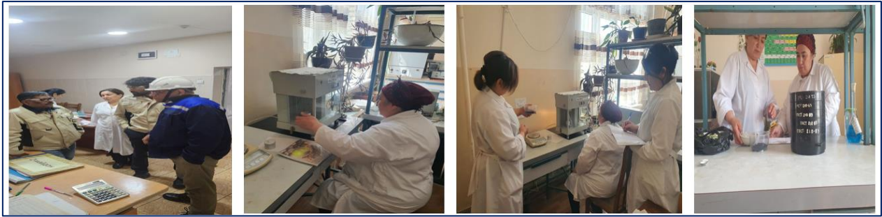
Figure -2 Weighing and sieving of Animal Bone char
