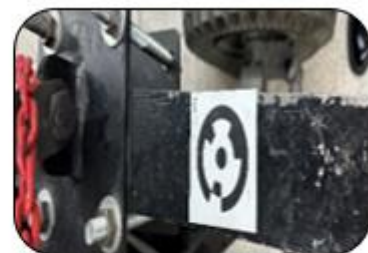
A point determination process has been applied for scanning the F4 engine.
