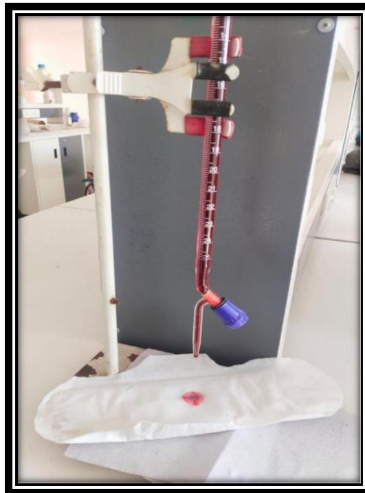
Fig24: Fluid absorbency test
