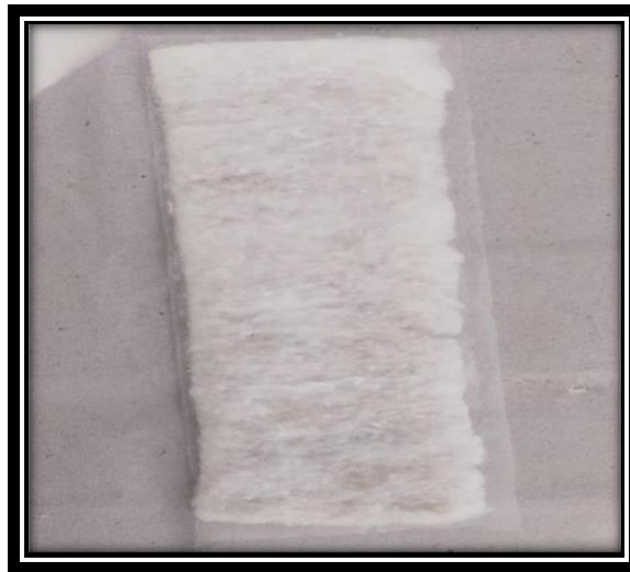
Fig16: Absorbent core + non-woven sheet (Middle layer)
