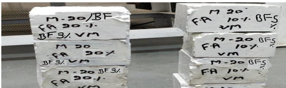
Figure 3: Specimen prepared after cutting and coated with epoxy.
