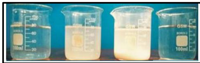
Fig -2.4: Preparation of MgO/water nanofluid.
