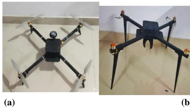
**Figure 4: Integrated drone-gripper system showing: (a) frame-gripper mounting interface (b) mainframe connection**
