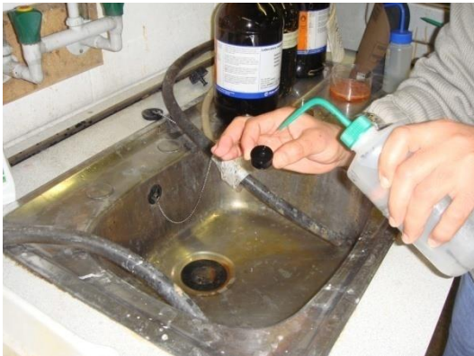
Fig 4: The Specimen is washed with the Acetone and Remained to Dry
