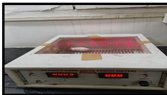
Fig 03- Determination of locomotor activity using Actophotometer
