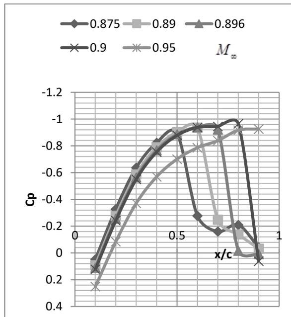
Figure 9. Pressure coefficients on upper surface at Tip station-Effect of increasing Mach number
