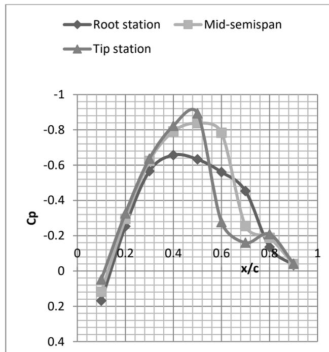
Figure 7. Pressure coefficients at  $M_{\infty} = 0.875$
