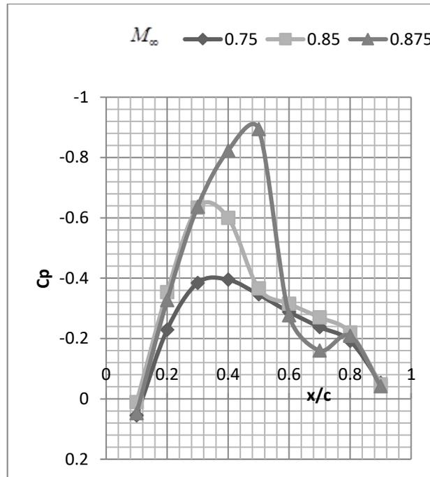
Figure 6. Chordwise pressure coefficients
