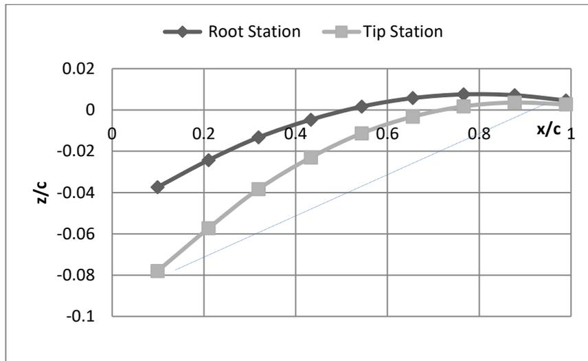
**Figure 3. Chordwise variation of vertical ordinates of optimal wing, M<sub>∞</sub>=0.75 and alpha = 4°**
