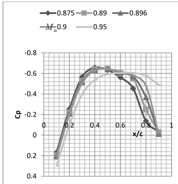
**Figure 10. Pressure coefficients on upper surface at Root station-Effect of increasing Mach number**
