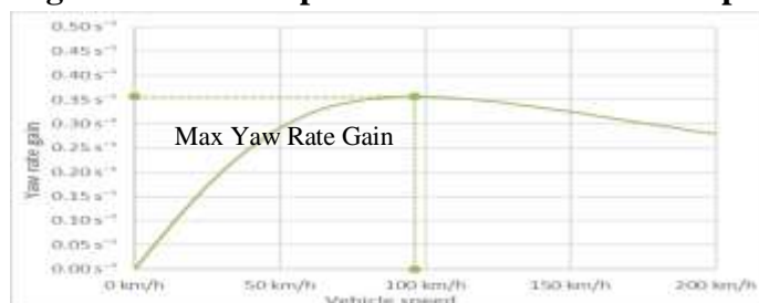
Figure 6. Vehicle Speed vs Yaw Rate Gain Graph.
