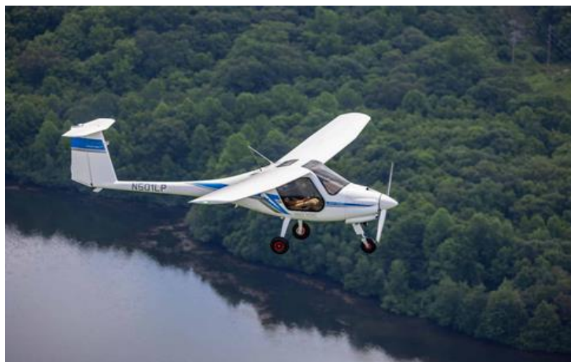
Figure 2 illustrates Pipistrel's Alpha Electro—the first electric aircraft used for flight training—highlighting the practical application of emerging electric propulsion technologies in lightweight aviation. (Pipistrel, 2021)
