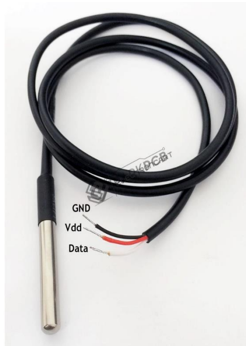
Fig 4:DS18B20 Temperature Sensor
